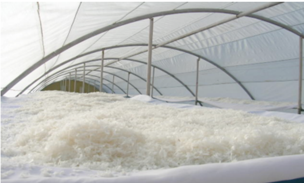
Figure: Shrimp-derived chitosan drying in a greenhouse. Picture: Dominique Gillet.
